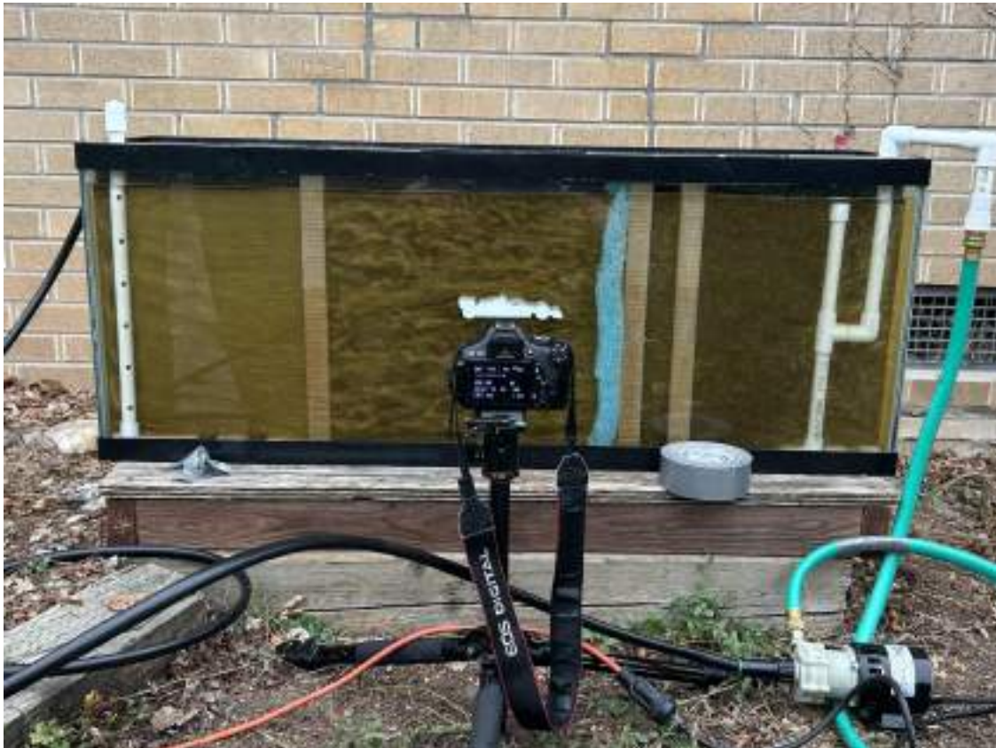
Figure 2: Water Tunnel and Camera Setup
